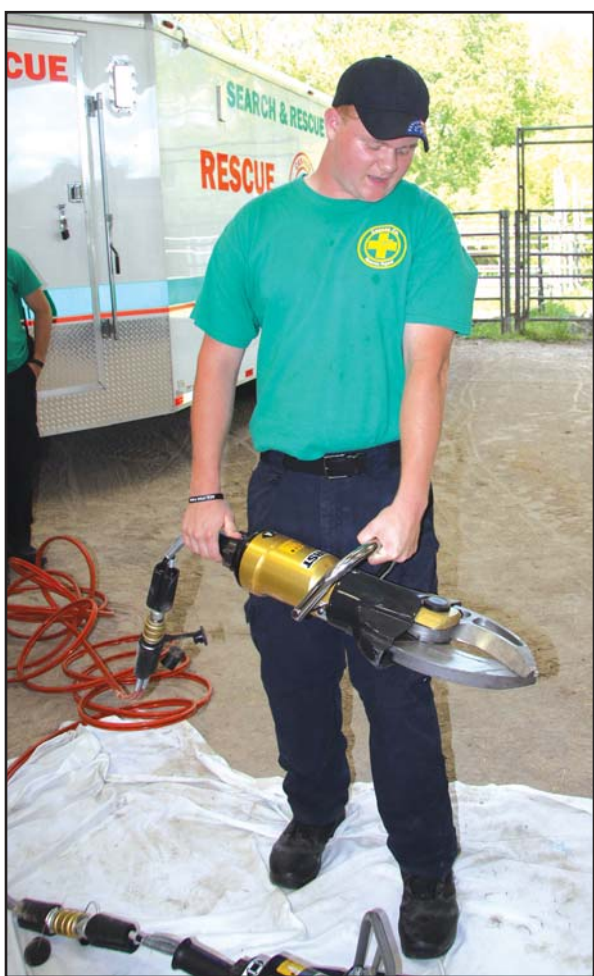
MIKE WEST photo Junior Rescue Squad volunteer Will Daniel demonstrates the Jaws of Life. The new jaws operates at 10,000 psi and is designed to cut through boron steel.
